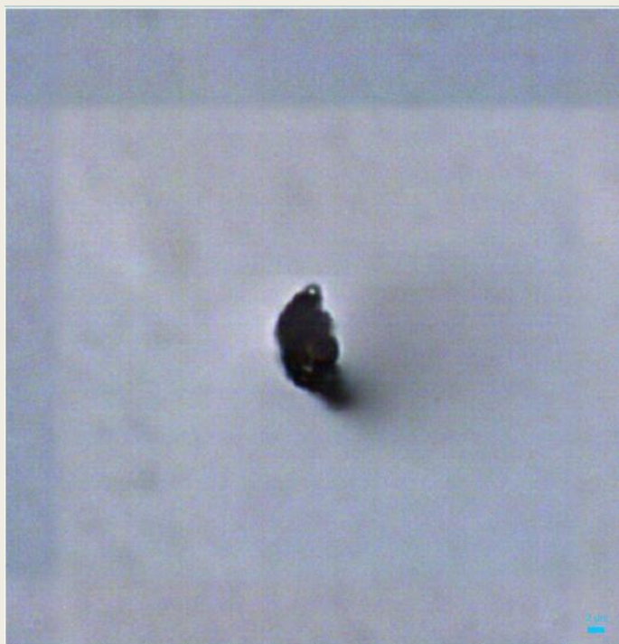
▲ Graphene-like particle image acquired with transmitted light and 100x objective
